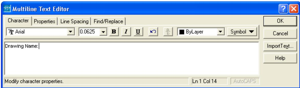
Figure 9.6 – Set the Text to 0.0625 Height and Type “Drawing Name:”
