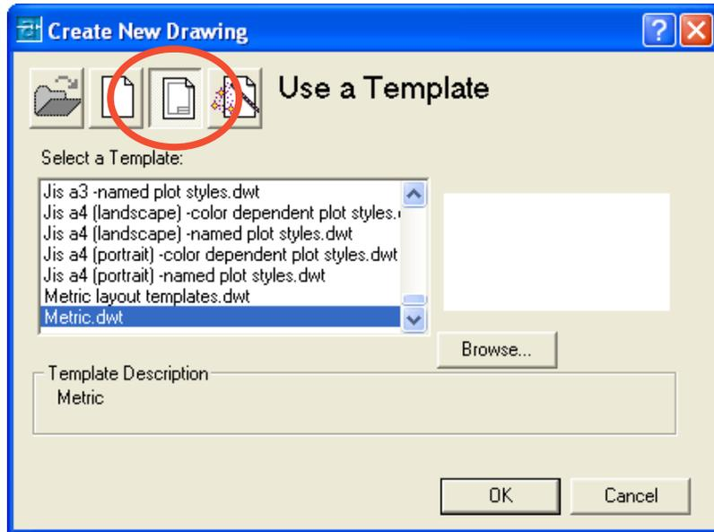
**Figure 9.3 - Starting the Drawing Using the Mechanical Template**
