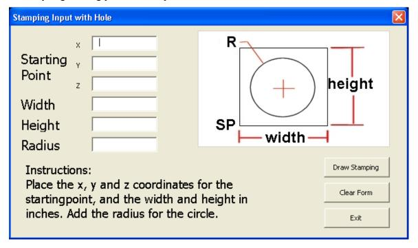
Figure 18.8 – Visual Basic Application Program Form for Drawing a Stamping
