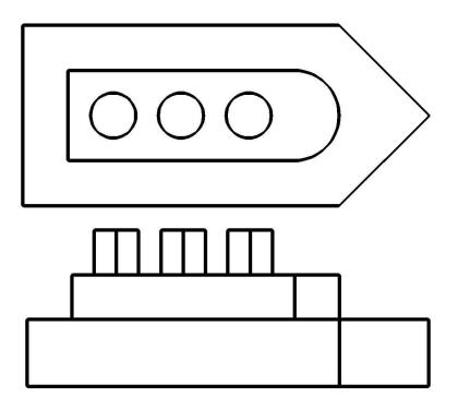
For all we know, the boat could be an inch to 10 feet long. To show the exact measurements, you will need to add dimensions to the drawing.
