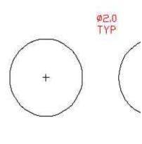
When placing radial dimensions on the sketch, first write the measurement relatively close to the object. For diameters, use a "0" sign in front of the dimension. For a radius measurement, use an "R".
