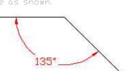
Next, draw two lines from either side of the angle measure, creating an arc. Place an arrow at the end of each line. The arrows should be perpendicular to the edge to which they are pointing.
