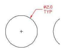
Next, draw a line to the object and place an arrow at the end. The arrow should be pointing at the center of the circle or arc. In this instance, the line is bent to face the center.
