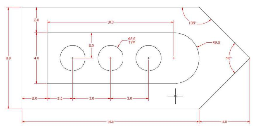
There are three types of dimensions shown above: linear, radial, and angular. Linear dimensions show length, like the 14.0 unit measurement along the bottom of the drawing. Radial dimensions show the size of circular elements measured from or across the center point, like the 2 unit diameter smokestack. Angular dimensions show angles between lines, like the 90° point on the front of the boat. All these types of dimensions are drawn with a different format.
