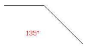
To place an angular dimension, first write the angle measurement in the center of the angle as shown.
