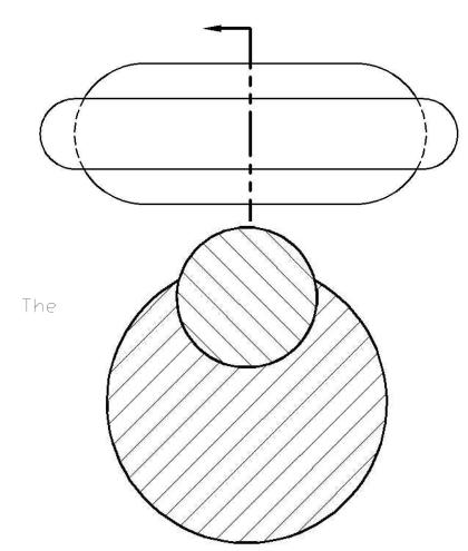
Above is the sectional view defined by the cutting line in the drawing to the left. As you can see, it looks very similar to the right side view drawing, except for the diagonal lines running through the middle. These lines are called HATCHING LINES and are used to define different types of materials. As there are no specific hatching patterns to show hot dog meat or bun, the two sections are hatched with the standard pattern for any material.
