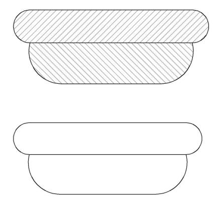
Pictured above is the same sectional view of the hot dog. Practice drawing your own hatching lines using the outline above, referring to the view in the bottom left-hand corner of the page if you have trouble.
