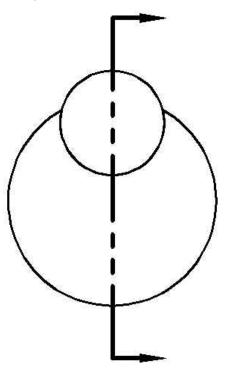
Here is another example of a sectional view. To the left is the right side view with a cutting line splitting the hot dog down the center. Below is the sectional view of the hot dog, complete with hatching, Though the bun does wrap up around the hot dog on the outsides, those details have been omitted. Had they been included, they
