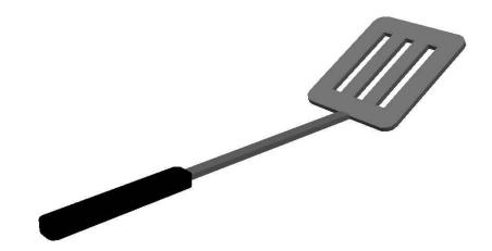
The spatula is an unusual object in that even if it is drawn using all six orthographic views, the drawings cannot be dimensioned correctly. Because the face of the spatula extends at a different angle from the handle, an auxiliary view is required to show the face straight on in addition to any other necessary views.
