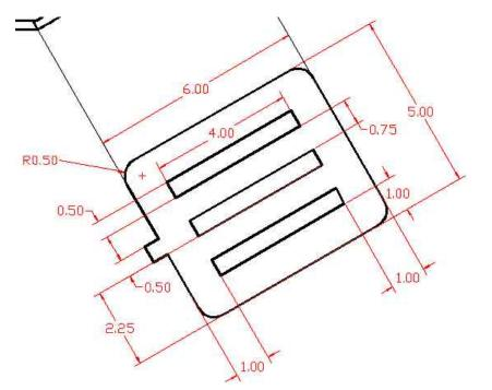
Here is the dimensioned auxiliary view. Notice how the dimensions are placed aligned with the drawing.
