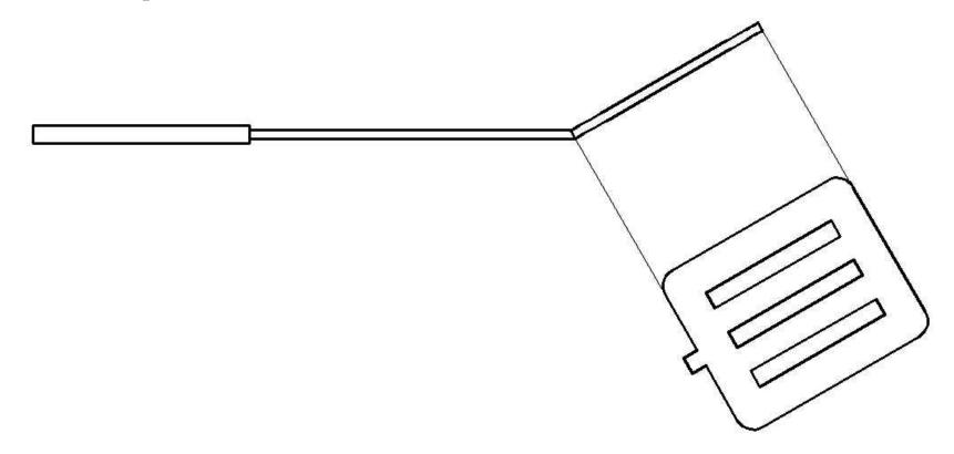
Here is the spatula with the auxiliary view. To draw the auxiliary view, draw two extension lines coming off of the face at the same angle. Now you can draw the view straight on, using the extension lines to align the view.
