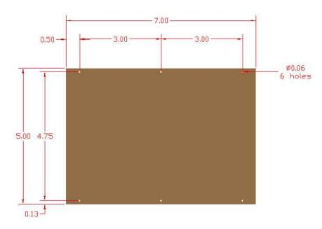
Let's start with the bottom. As you can see in the picture above, the bottom of the box is 5" by 7". Also, it has six 0.06" holes placed around the outside.
