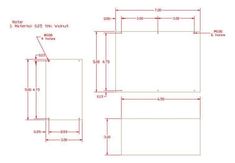
Here is a picture of the finished assembly drawing. The pieces are shown from the top view and laid out near the edges where they will be attached. Only one side from each of the pairs of sides is shown. In addition, a Notes section is included in the top left-hand corner showing the material used.
