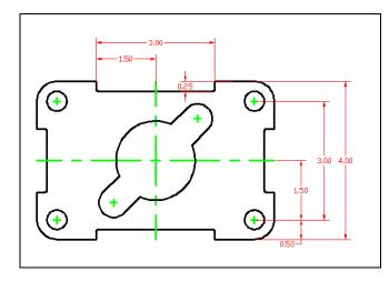
Continue to use the Linear Dimension command by pressing ENTER each time to repeat the command. Always dimension from the inside to the outside of the part, so you always have room for more dimensions. Do the 1.50, the 3.00 and 4.00 dimensions trying to space them evenly (Figure 3.18). To place the 0.50 dimension, select the right of the 0.50 centerline and the part. For the third selection to show position, select the 1.50 dimension line. The dimension lines will line up.
