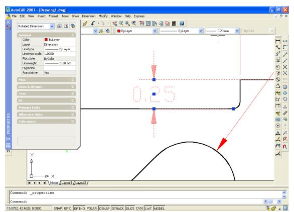
Figure 3.32 - Using the Properties window to remove a dimension extension line
