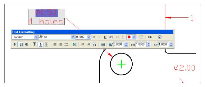
Figure 3.37 – Adding text to a dimension
