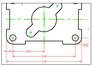
**Figure 3.19 – Dimensioning the bottom**
