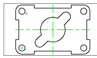
**Figure 3.10 – Placing center marks**
