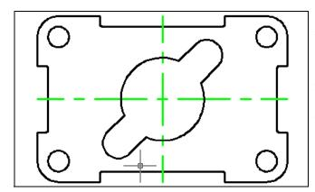
The Center layer replaces the 0 layer to show that these two lines now reside on the Center layer. Press the ESC key on your keyboard and the lines are no longer dotted and are removed from the selection set. Centerlines are critical in the dimensioning process since they show symmetry in a part and reduce the amount of dimensions on the drawing. When an reading prints, clarity improves the communication process.
