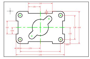
Place the last two dimensions on the left side of the drawing, doing the 0.80 dimension first and the 1.60 dimension second. There are 13 linear dimensions on this part.
