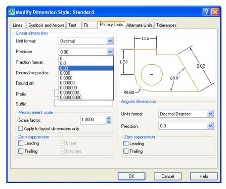
Select the Primary Units tab to change decimal places. The form is broken into Linear **Dimensions and Angular** Dimensions halves. In the Precision list box in the Linear Dimensions select section. the dropdown menu to open the list and highlight the 0.00 in the list to change from 4-place to 2-place decimal. In addition, vou can change the Precision in the Angular Dimensions list box to 0.0 (Figure 3.15).
