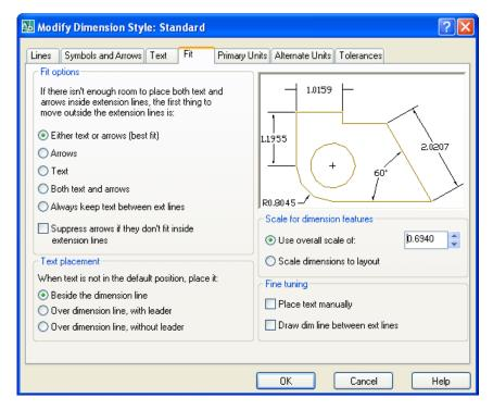
There are 6 tabs in the Modify Dimension Style window<sup>.</sup> Lines and Arrows, Text. Fit. Primary Units, Alternate Units, and Tolerances. You need to select the Fit tab and change the scale overall of dimension from 1.0 to (Figure 0.694 3.14). There only is one textbox in this window, so it is easy to locate and make the change.
