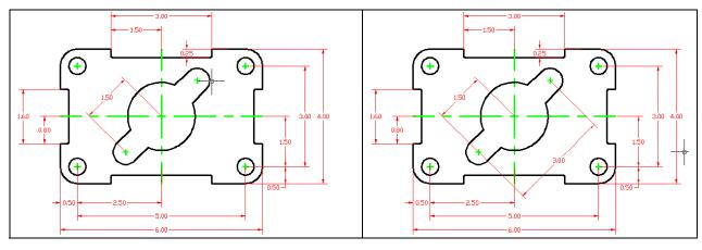
**Figure 3.21** – 1<sup>st</sup> aligned dimension
