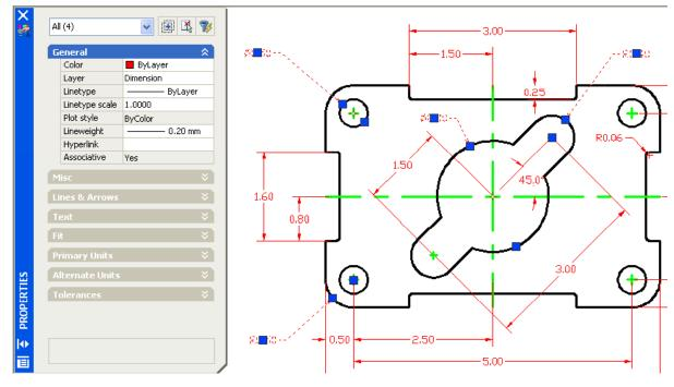
Figure 3.35 – Turning off the Center mark on four dimensions
