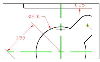
The second diameter you will place on the drawing is on the 2.00 diameter hole in the center of the part. Select the Diameter Dimension tool on the Dimension toolbar and the aperture cursor will change to a pick box. Select the 2.00 circle. Make your second selection to place the dimension text on the drawing (Figure 3.28).
