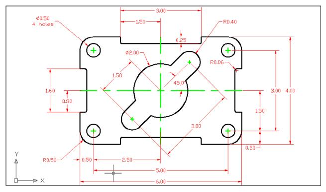
Figure 3.38 – Finished dimensioning the rectangular problem
