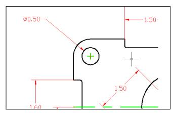
Select the Diameter Dimension tool on the Dimension toolbar and the aperture cursor will change to a pick box. Select the 0.50 circle located on the upper right hand corner of the part. Similar to the Radius Dimension command, a second selection will place the diameter text on the drawing (Figure 3.27).
