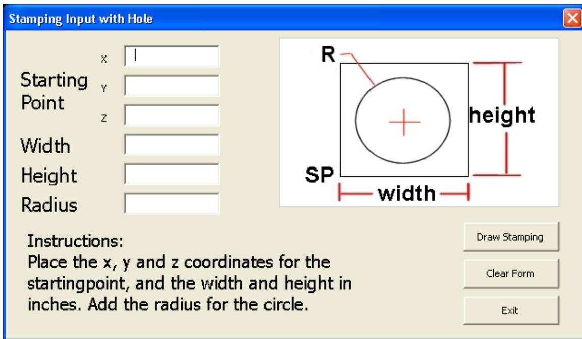
Figure 18.8 –Visual Basic Application Program Form for Drawing a Stamping
