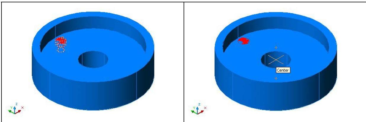
Figure 14.32 –Center of the Polar Array
