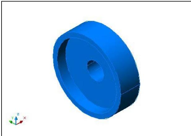
Select the Shade tool on the Shade toolbar. The part is now a solid blue color as shown in Figure 14.19. The tessellation lines associated with the Hide command are no longer interfering with your ability to read the drawing. Your customers will most likely prefer this mode to the Hide command since they can visualize the product clearly. If you ever desire to return to standard viewing, choose the 2D Wireframe tool on the Shade toolbar to return the drawing to the previous settings.
