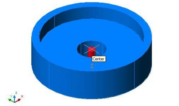
Figure 14.25 – Center of Second Cylinder
