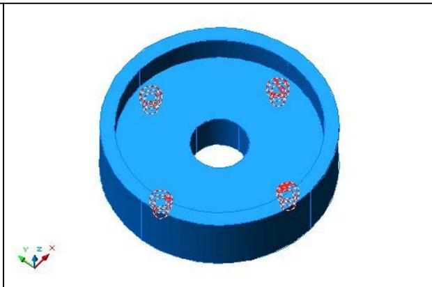
**Figure 14.36 – Subtracting Solids**
