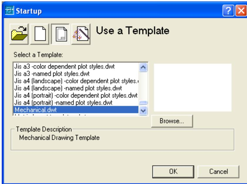
Figure 14.2 – Starting the Drawing Using the Mechanical Template
