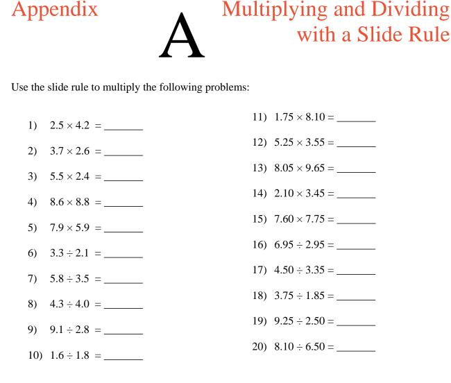
To multiply, we place the 1 on the upper scale overtop the first number in the problem on the lower scale. Now, we follow the upper scale until we read the second number. It is over the answer that is on the lower scale.
