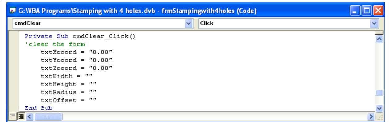
Figure 4.28 – Computing the Reset Button by Clearing Textboxes
